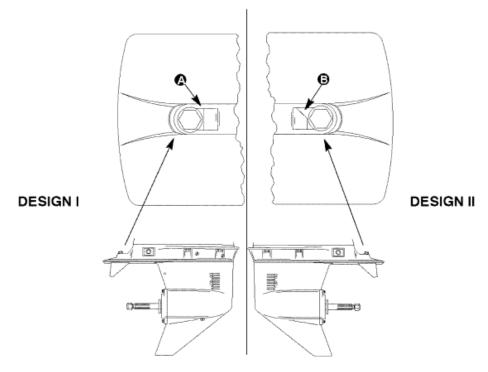
NOTE: TO INSURE ORDERING THE CORRECT REPLACEMENT GEAR HOUSING COMPONENTS, IDENTIFY YOUR GEAR HOUSING BY USING THE DIAGRAM ABOVE. IF YOUR GEAR HOUSING (DESIGN I - 3 JAW REVERSE CLUTCH) HAS A STRAIGHT MACHINED EDGE FOR TRIM TAB SCREW MOUNTING (A), ORDER FROM GEAR HOUSING BREAKDOWN PAGES (3 JAW REVERSE CLUTCH). IF YOUR GEAR HOUSING (DESIGN II - 6 JAW REVERSE CLUTCH) HAS AN ANGLED MACHINED EDGE (B) ORDER FROM GEAR HOUSING BREAKDOWN PAGES (6 JAW REVERSE CLUTCH).
